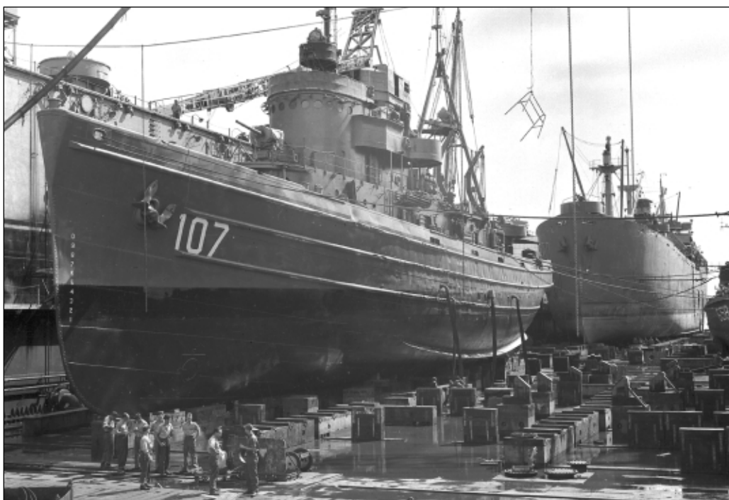
This photograph shows the U.S.S. Munsee, ATF-107, in an Advance Base Sectional Drydock (ABSD) at Guam for repairs in July 1945.
